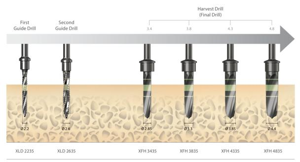
\* During the 4.3/4.8 fixture insertion into the bone density of D3~D4, the 3.35/3.85 harvest drilling process can be skipped.
