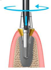
Rotate the tool counterclockwise until tightly locked into the 1.28 hex of the abutment screw
